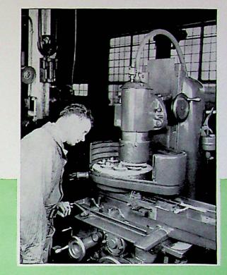
0.04 mm. at each table reversal. The dial can be set to a predetermined depth of cut and will automatically throw out the feed at the desired point, or it can be locked for continuous feeding. Wheel wear must be considered when working to close figures.
