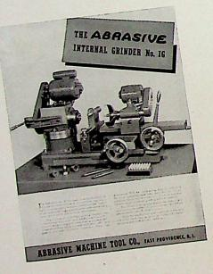
The Abrasive No. IG Internal Grinder has been developed recently to handle the large volume of manufacture requiring a highly accurate, easily handled, internal grinder. Typical of such work is the huge quantity of die work, particularly those used in bullet and cartridge manufacture.
