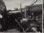
Head and tailstock Spindle alignment, straight to .001 high on tail.
