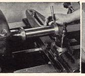
Boring test, 8" bar with collars turned and "miked" to straight with .0005 large at outer end.
