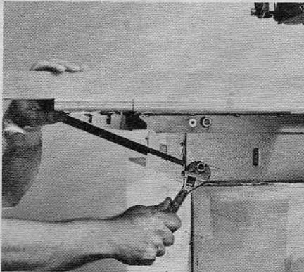
11. Lay spacer board on table top. Hold table extension parallel with table top, adjust and tighten support nut and bolt.
