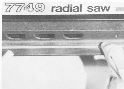
5. To install motor assembly, first, back out the two set screws on end cap sufficiently to allow the paddle to be lifted and held in a position to remove the end cap mounting screws.
