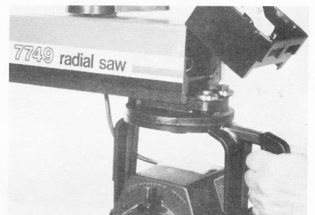
6. Carefully slide the motor assembly into arm. Replace the end cap and tighten mounting screws securely. Check to be sure the shroud is assembled properly in the front and rear end caps. Without "Power" pull the motor assembly forward firmly against the front end cap. The end cap should stop the motor assembly with no apparent movement. If not, check the front end cap mounting screws and tighten these screws securely.
