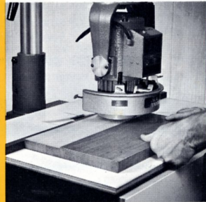
It's a SURFACER . Rotary planer tool fits directly on motor spindle . . . smooths out rough lumber, gets it ready for sanding.
