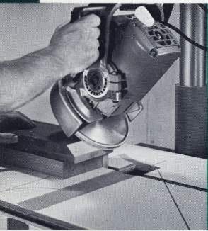
BEVEL SANDING • Put Disc Sander into bevel position and pull across the stock setting on a fixture . . . the only sander that does this.
