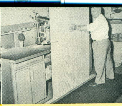
HORIZONTAL SAWING. Tilt motor vertical, set saw parallel to table top and cut across 4 foot wide panels this way. Saw can be lowered or raised for desired width.
