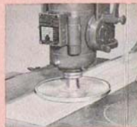
TILTING ARBOR DISC SANDER Tilts any angle, usable many ways, work lies flat on table.
