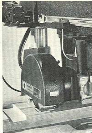
Optional accessories convert saw to a dado machine.
