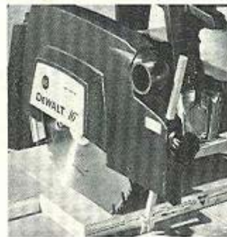
Blade guard has anti-kickback device. Built-in metal dust chute.
