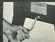
Up Front elevation control. Precision depth adjustment as fine as \frac{1}{16} ".
