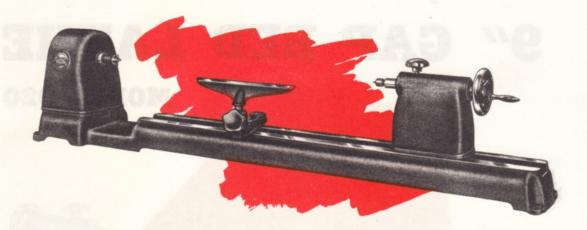
Darra-James Model 920 is a sturdy fine grain cast iron lathe offering four speeds. The rugged tailstock glides easily on accurately machined ways. Ground steel spindle is threaded both ends for outboard turning. Swing over bed is 9" with 11" over gap. Tail stock center is self-ejecting. Oilite bronze bearings mean long trouble free service.
