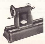
Screw-type lock saves time in positioning tailstock. All locks on lathe alike. No wrenches necessary. With a substantial lathe, wood turning is one of the most fascinating — and one of the easiest — of all wood working operations. If it is an art, it is largely the art of a competent machine.
