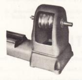
Big headstock cast in one piece with open back to permit easy access to spindle pulley. No hood, no hinges.
