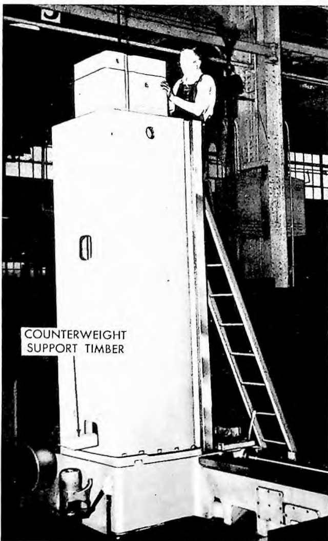
Figure 5. Lowering Counterweight into Column
