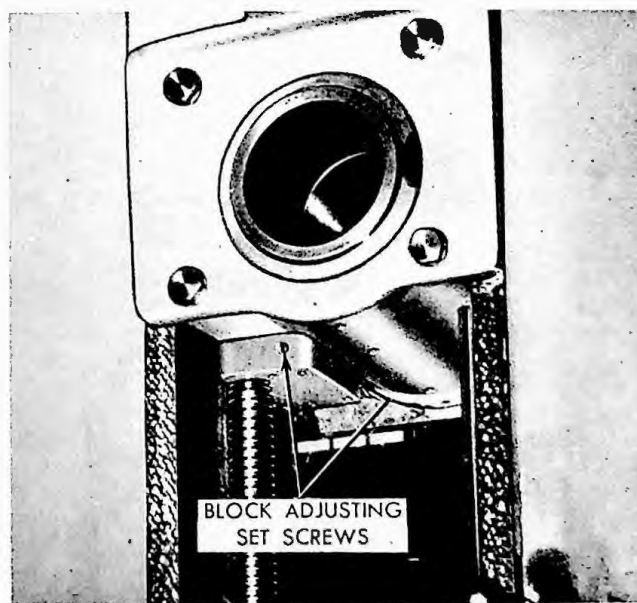
Figure 40. End Support Bearing Block Adjustment
