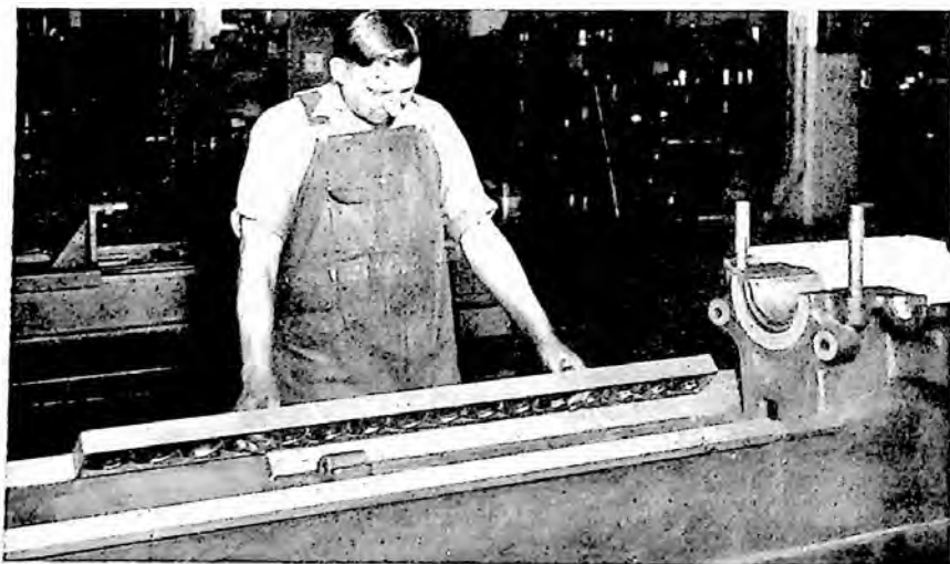
Fig. 2—Straight-Edge Used in Re-Scraping Turret Lathe Bed
