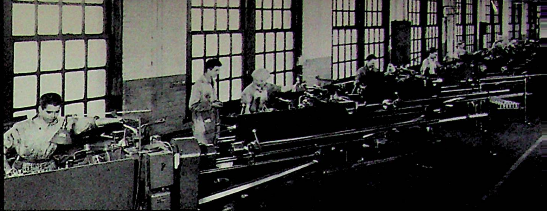
FIG. 2 Proper location of Turret Lathes on upper floors near wall
