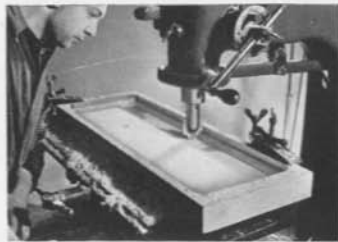
The machine is exceptionally useful for panel sinking operations as shown above.
