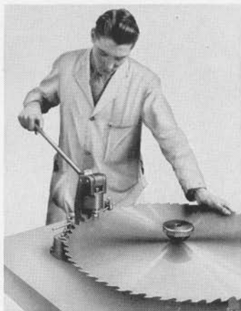
With this Wadkin Circular Saw Setter it is an easy matter to leave every tooth uniformly set to a specified amount
