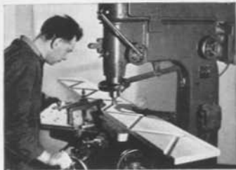
Cutting housings for string boards. Fixture in use dispenses with the need for marking out.
