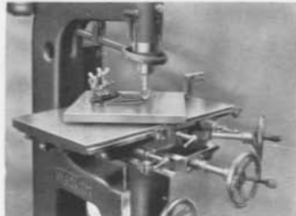
Circular moulding can be done by means of auxiliary rotating table.
