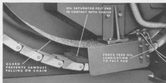
Shows the method of lubricating the chain.
