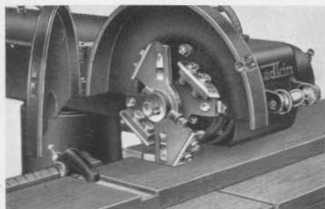
Saws can be taken off, and this expanding grooving head substituted in two or three minutes
