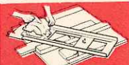
Saw guide pivots on clamp bolt to allow miter and compound cuts
