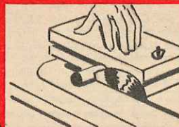
Metal Cutting . . . use cut-off wheel in place of blade
