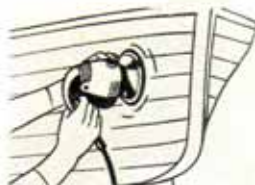
Flexible sanding discs are just the thing for sanding curved or irregular work surfaces
