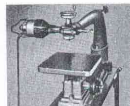
Router head assembly tilted for spindle carving. Spline on head shows angle of tilt.
