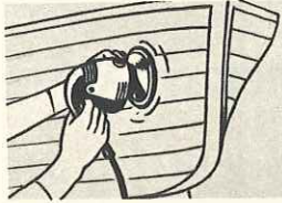
Flexible sanding discs are just the thing for sanding curved or irregular work surfaces
