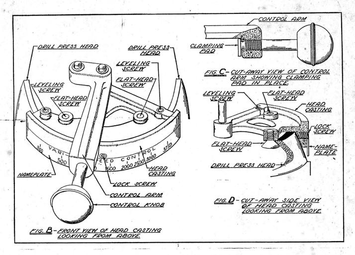
B & D. Caution: Do not tighten Leveling Screws so much that the Flat-Head Screws are raised out of place.
