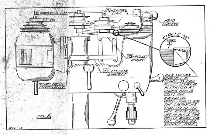
The Vari-Slo Speed Control attachment, when properly installed on either of the above listed drill presses, slows the original lowest speed of 625 R.P.M. down to 300 R.P.M. and gives any speed desired from 300 R.P.M. to 3750 R.P.M. quickly, with no belt changing. The operator can read the correct spindle speed directly from the indicator dial, and can change the R.P.M. quickly to any indicated speed from 300 to 3750 R.P.M.
