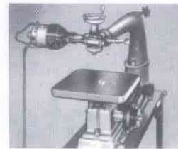
Router head assembly tilted for spindle carving. Scale on head shows angle of tilt.
