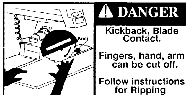
Fig. 3 Blade Contact Safety Sign
