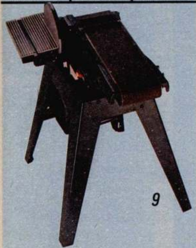
9 ¾-HP belt-disc sander* has over 100 sq. in. of sanding surface for sanding and finishing most straight and curved surfaces. Cast iron platen tilts and locks in horizontal and vertical positions. Belt travels approx. 2700 ft. per min. 9-in. disc rotates approx. 3450 rpm. Removable 6¼x12-in. cast aluminum table has ¾x¾-in. groove for miter gauge. Incl. steel stand, med. grit sanding disc and a guard with 2½-in. diam. coupling for use with vac. Capacitor-start induction-run belt-drive motor. 6-ft., 3-wire cord. Unassem. 9 R 22593N—Wt. 133 lbs . . . $379.99
