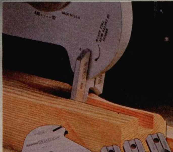
Carbide-tipped adjustable dado features hub to let you dial any width from 3/16 to 13/16-in.!
