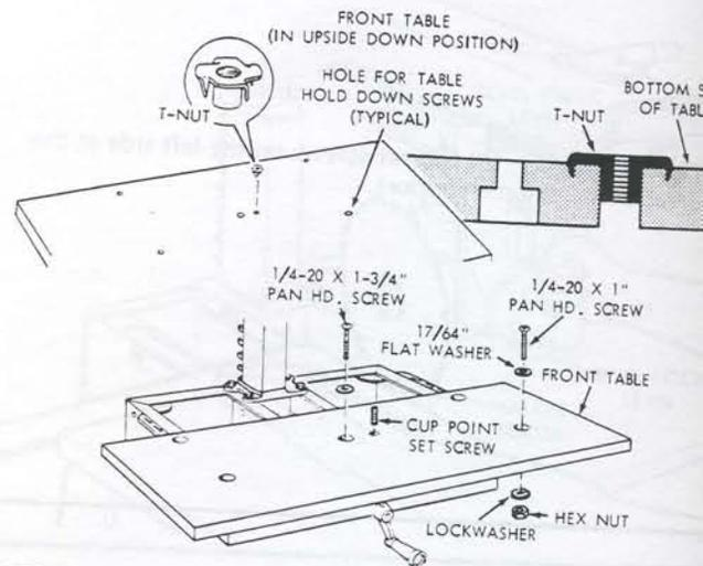
4. Lay the rear table board on edge across the front table to serve as a straightedge. Sight under this straightedge to determine whether the front table board is high or low at its center.
