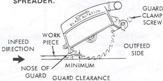
1. The blade guard is positioned by loosening the guard clamp screw and rotating the guard so that the nose just clears the workpiece as shown.
