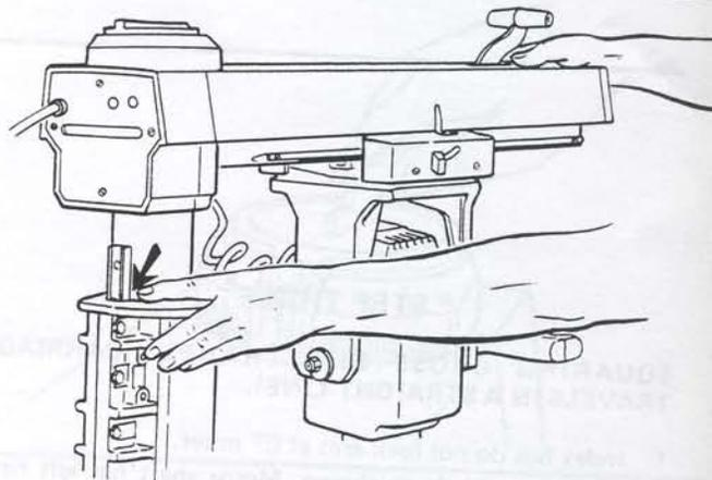
2. Remove Column Support trim using screwdriver as shown.
