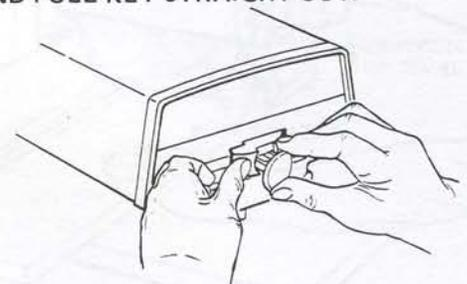
**WARNING: FOR YOUR OWN SAFETY ALWAYS LOCK THE SWITCH "OFF" WHEN SAW IS NOT IN USE. REMOVE KEY AND KEEP IT IN A SAFE PLACE . . . ALSO IN THE EVENT OF A POWER FAILURE (ALL YOUR LIGHTS GO OUT) TURN SWITCH OFF. LOCK IT AND REMOVE THE KEY THIS WILL PREVENT THE SAW FROM STARTING UP AGAIN WHEN THE POWER COMES BACK ON.**
