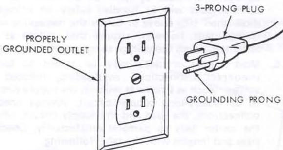
This power tool is equipped with a 3-conductor cord and grounding type plug which has a grounding prong, Listed by Underwriters' Laboratories. The ground conductor has a green jacket and is attached to the tool
