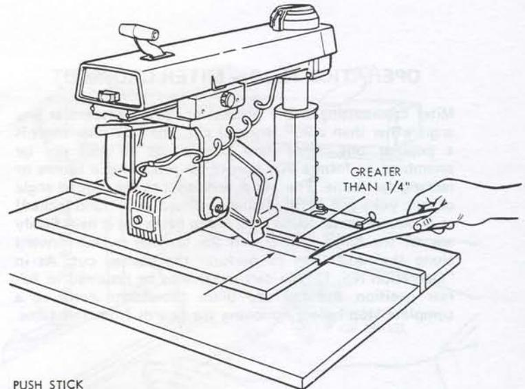
7. When ripping stock 1/4 inch or less between the blade and fence (guide) use a Pusher Board. Pusher board should not be less than 3 inches wide and 16 inches long. Nail or glue a 3/4 x 3/4 x 4 inch block to one edge of pusher board to be used as a grip. The pusher board should be fed into the blade behind the stock being ripped until the stock is clear of the rear of the blade (not more than 8 inches so as not to strike antikickback pawls) and then pulled back with use of the grip.
