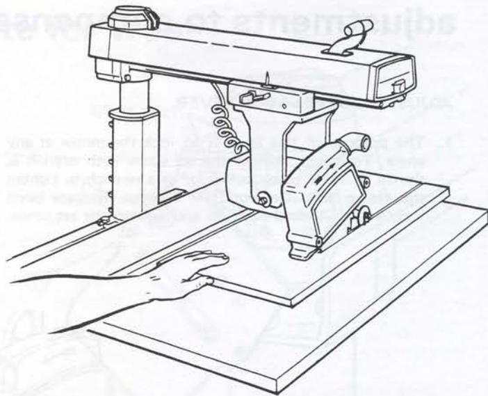
**In-Ripping.** The radial arm and bevel are indexed at 0° and locked, but the yoke is turned 90-degrees in a clockwise direction (viewed from above) from the crosscut position. Thus, when standing in front of the saw, the blade would be rotating counterclockwise. After positioning the guard and antikickback mechanism the workpiece is fed from the right-hand side of the saw. The "Blade In-Rip" scale is on the right-hand side of radial arm.
