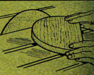
Sanding. For that "finishing touch," just replace saw blade with sanding plate
