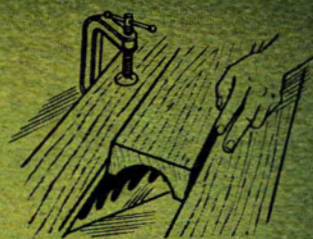
Cove cut. With proper blade, use to shape cove mouldings of various designs and sizes
