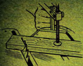
Compound cut. Saw at bevel angle and a miter angle for making tapered forms
