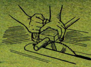
Metal cuts made with cut-off wheel. Also cuts concrete, plastic, brick or glass
