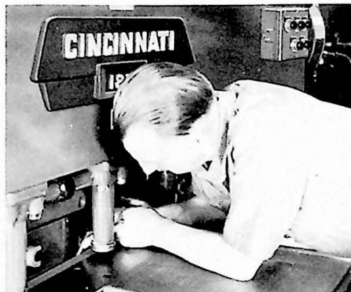
Fig. 21. Close-up of Knife Setting with Feelers
