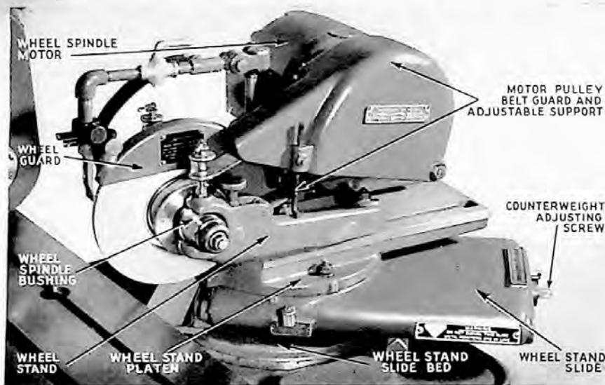
Fig. 4. Wheel Stand Assembly of the No. 1 Machine.
