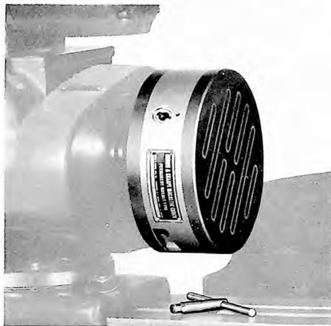
Fig. 35. No. 9R Rotary Model Magnetic Chuck (Permanent-Magnet Type), and Chuck Adapter Pulley in Position on the Headstock of a No. 2 Machine.
