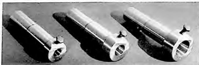
Fig. 33. Bushings for Holding Cutters with Standard Taper Shanks.
