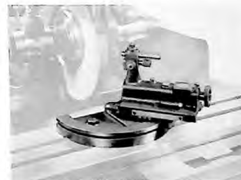
Fig. 28. Radius Wheel Truing Attachment.
