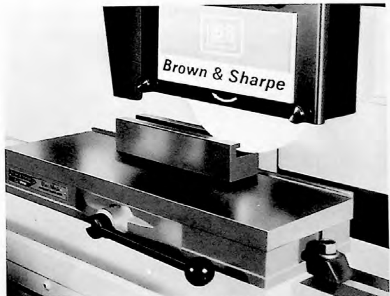
Fig. 2F. The table setting in fixed ways contributes immeasurably to slot and other forms of side wheel grinding.
