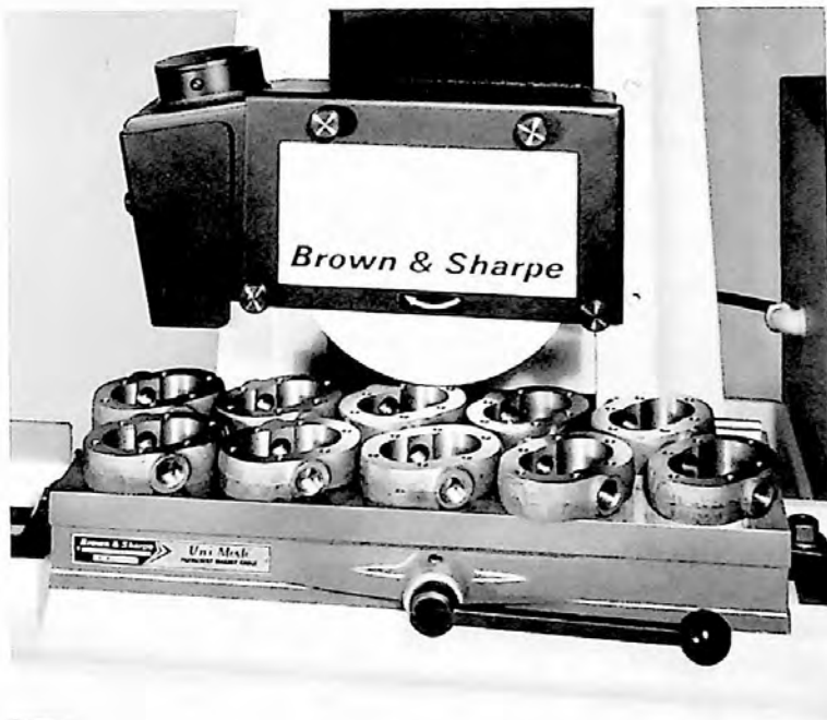
Fig. 1F. A representative production job, grinding the surfaces of ten pieces with one loading of the chuck.
