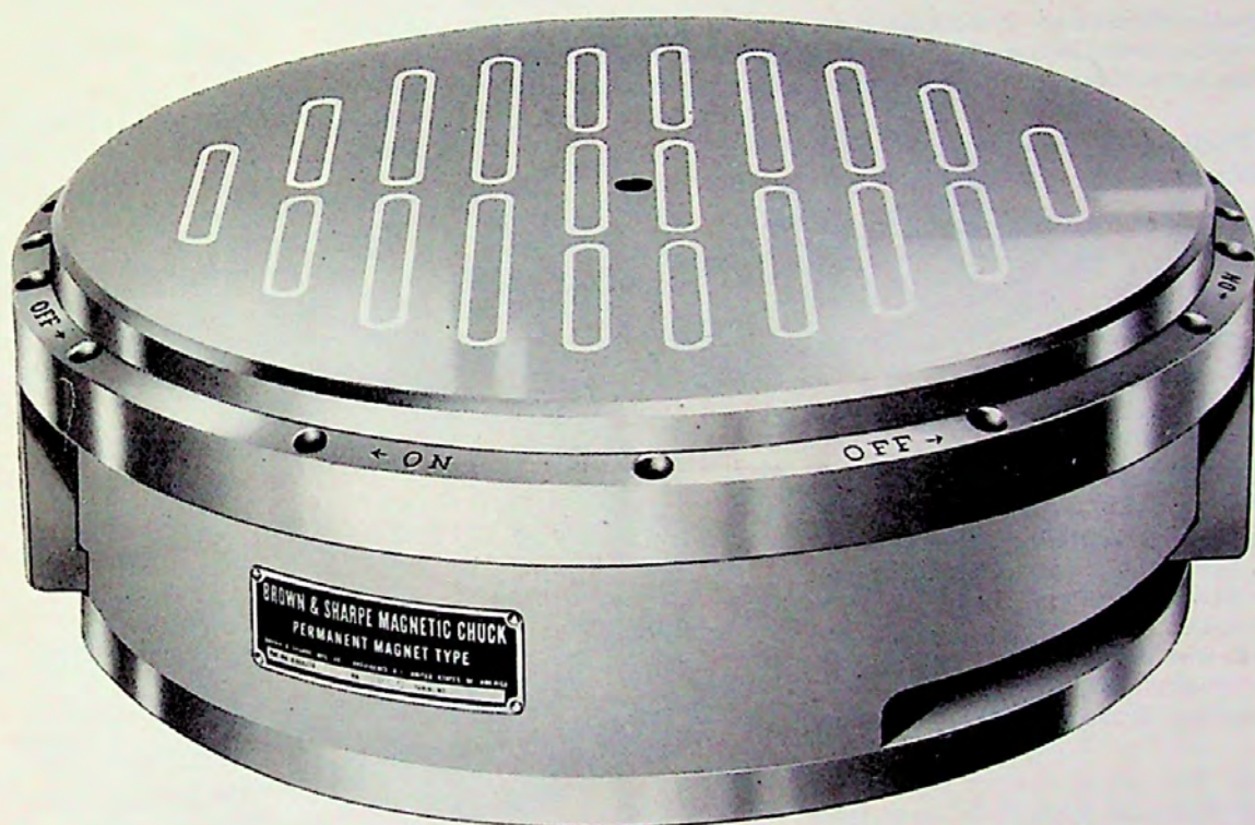
Large Rotary Chuck 16" in diameter. Chuck can be operated in any position by means of an operating pin inserted into any one of the holes of the control ring.
