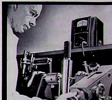
This measuring machine checks electronically the dimensions of plug gages. Measurements are made easily and read positively from the widely spaced amplifier dial graduations.
