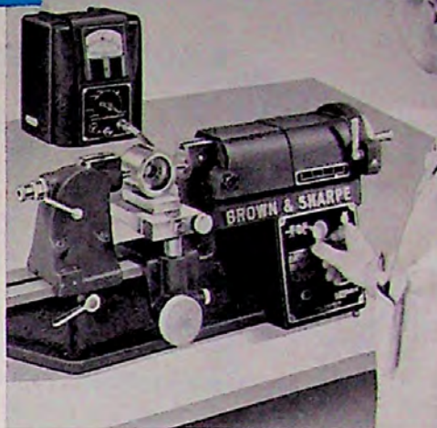
Measurements as close as .00001" are made easily on this machine with an 18,000 to 1 magnification—one of the many devices that maintain the high degree of precision in Brown & Sharpe Tools.
