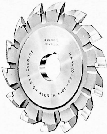
Carbide Milling Cutter for machining bevel on type metal plates. Plates are hot at time of machining.
