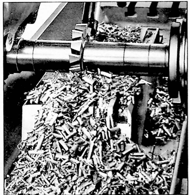
Staggered Tooth Side Milling Cutters with their alternate right-hand and left-hand spiral angles and deep angle of undercut provide a free cutting action that permits their employment for deep cuts which would stall an ordinary cutter. The illustration shows a typical example of deep slotting with the cutting efficiency indicated by the chips.
