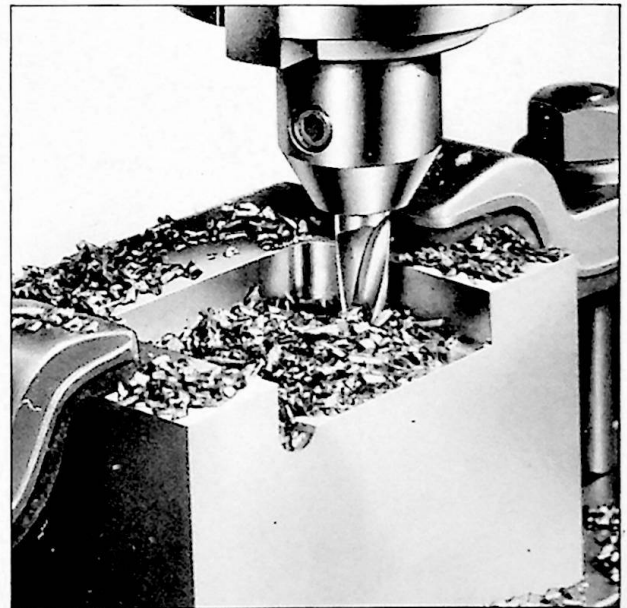
Ball End, Two-Flute Fast Spiral Single-End End Mills simplify the milling of slots or other surfaces requiring bottom radius or fillet, as shown in the illustration.
