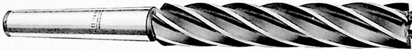
End Mill 1¾ inches in diameter and 18 inches in over-all length. Has 6 teeth with hollow faces and a 30° spiral.
