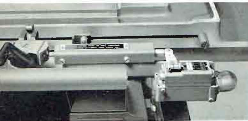
Below—Table reversing lever in contact with plunger causes spindle to feed down predetermined amount.
