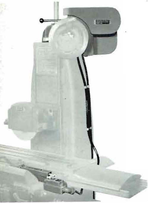
Above—View showing Spindle Power Down-Feed Arrangement on machine.
