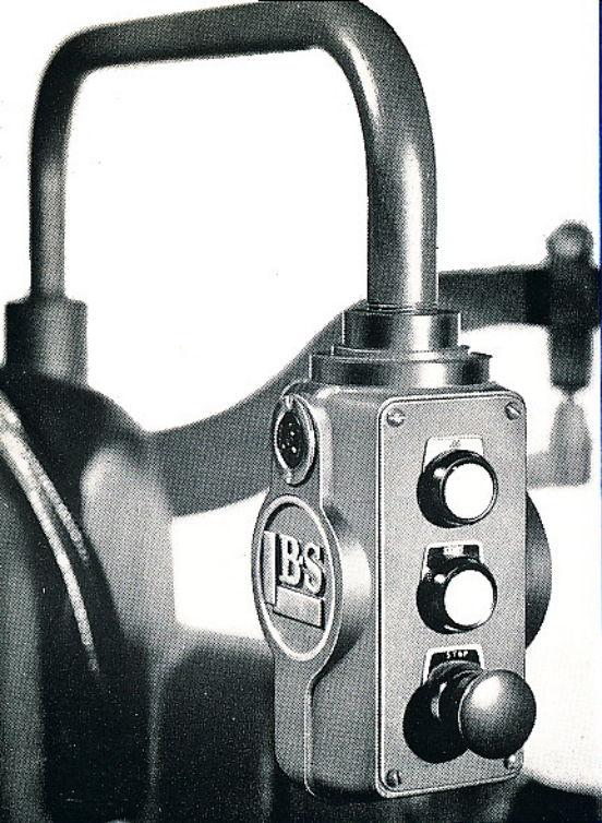
Spindle "Start", "Stop" and "Jog" buttons located on panel adjustable horizontally to most convenient operating position.
