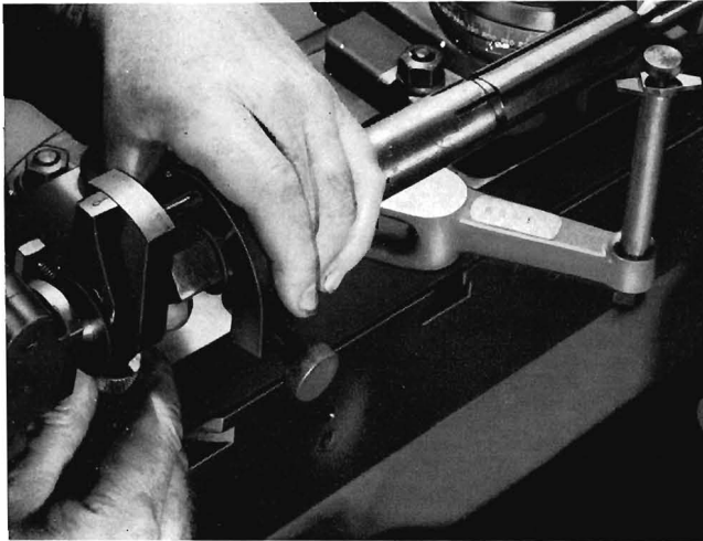
Fig. 6. Setting clearance angle for sharpening reamer using the Clearance Setting Gage.
