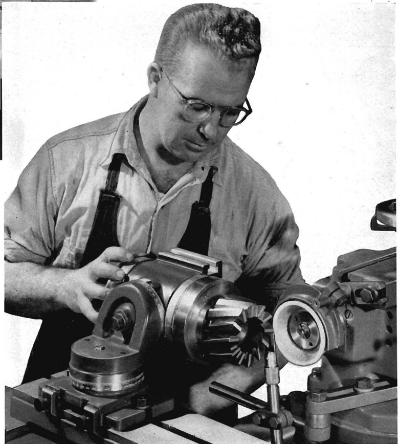
Fig. 22. Operator grinding the secondary clearance angle of a shell end mill using the rear table operating position. The cutter is mounted on an arbor held in the work head. Since a cup wheel is being used, tooth clearance is obtained by swiveling the work head. The tooth rest is mounted on the wheel spindle head with the blade in contact with the tooth being ground. Indexing for the next tooth is accomplished by simply turning the work head spindle.
