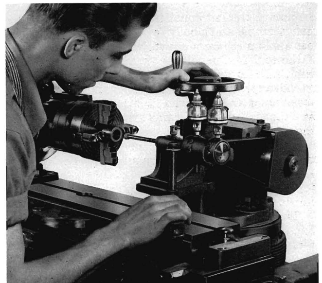
Fig. 7. No. 10N Internal Grinding Attachment being set to center height of work with the center gage.
