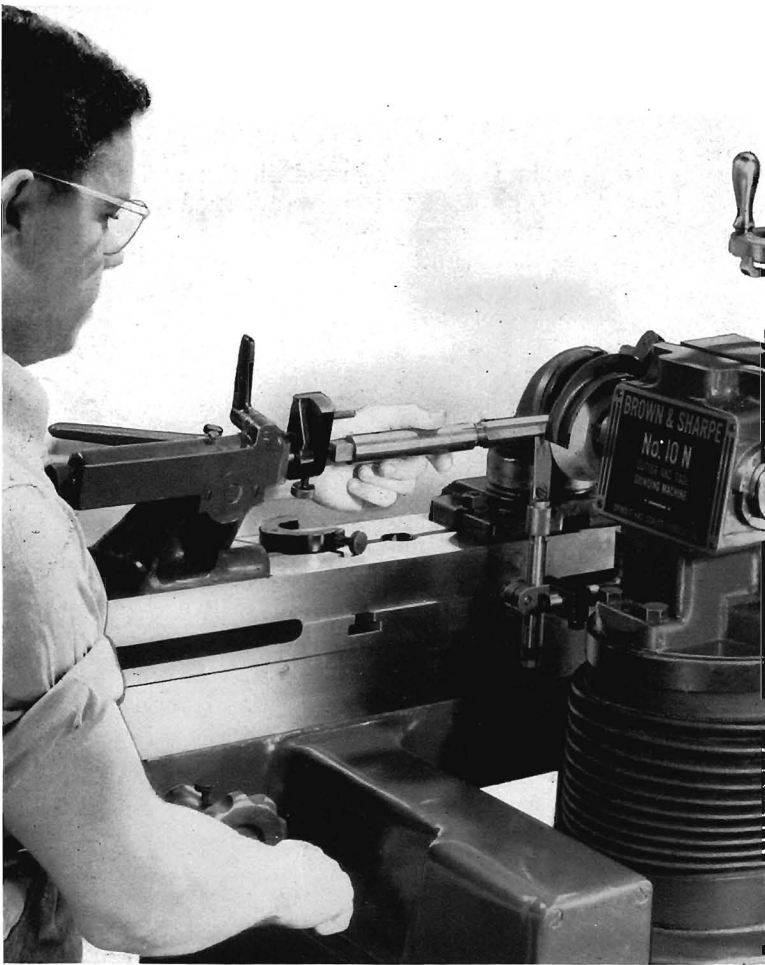
Fig. 23. Sharpening a straight finishing reamer. The reamer is mounted between the centers of the center head and footstock. The cup wheel is positioned so there will be no interference with the center head and proper clearance is obtained on the cutting edge of the reamer by using the center gage and the clearance setting gage when adjusting the height of the tooth rest. Table movement is by handwheel from the rear-of-table operating position where the sharpening operation can be most easily observed.
