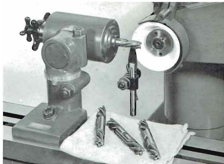
Above—Double-end end mills are quickly and easily sharpened on this Attachment. A spring collet and draw-in bolt are used to hold this type of cutter in the Attachment spindle.
