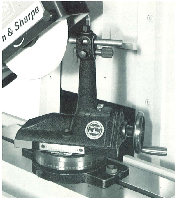
Fig. 10I. Shaping a radial contour with Radius and Angle Wheel Truing Attachment. The slide is clamped at the required radius, the diamond tool is set by the gage just below it and the slide is swiveled to form the wheel.
