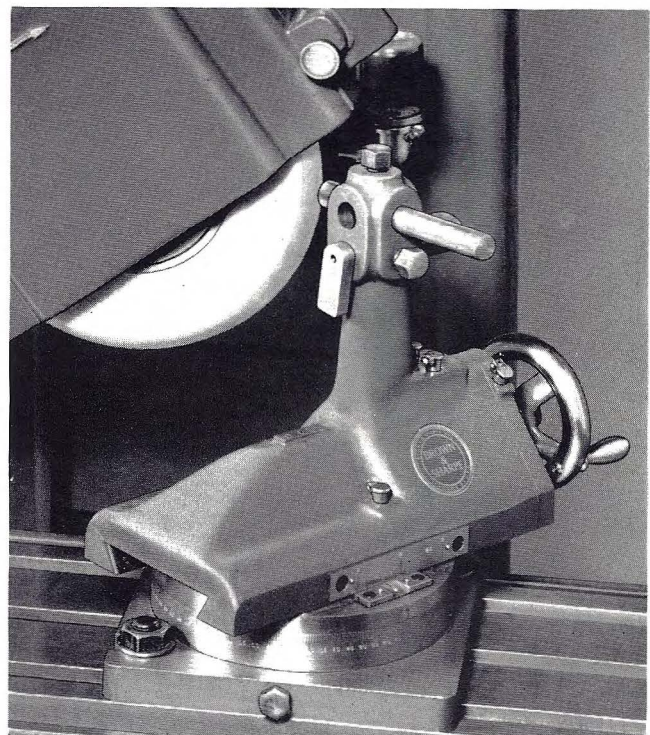
Fig. 29. Forming an angle. The swivel platen is clamped at the required angle and the slide is operated by the handwheel to true the wheel. In both cases the diamond is advanced by hand feed of the machine table.
