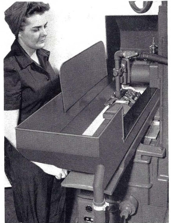
Fig. 22. Wet Grinding Attachment in use, showing adjustable splash guard on rear of work tank and removable splash guard on front.
