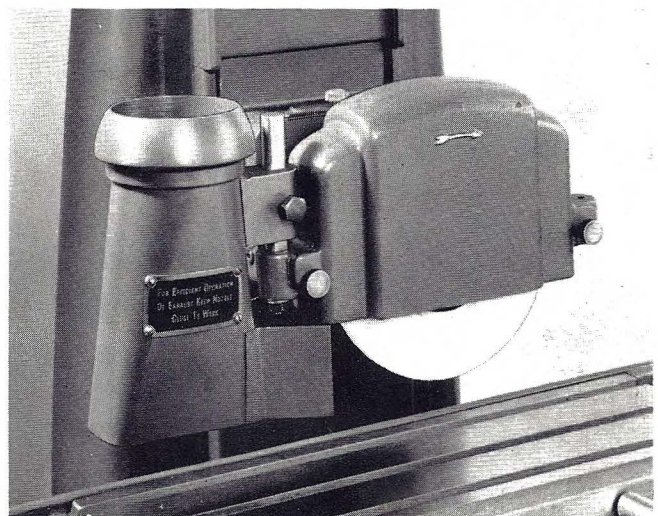
Fig. 20. Nozzle for connection to plant exhaust system.
