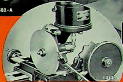
CLOSE-UP OF JOB— GRADUATING 1 3/8" DIAL With Automatic Indexing Controlling Accuracy of Spacing and Varying Length of Lines.
