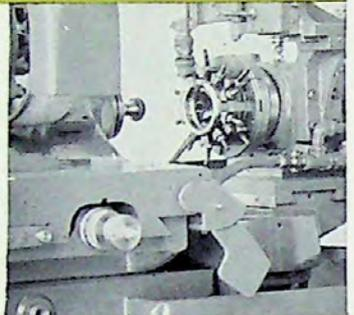
Grinding a thrust bearing.
