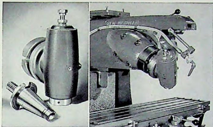
The Universal Subhead increases the usefulness of Van Norman Ram-Type Milling Machines in three basic ways:
