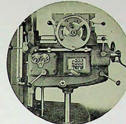
Front and rear control of hand and power feeds give complete visibility and control of operations from either location. Reduces worker fatigue . . . improves work accuracy.
