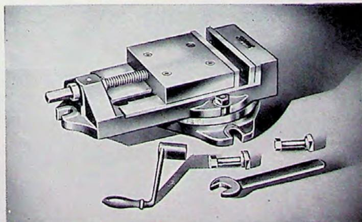
Van Norman Vises are designed for maximum utility and durability. They are precision-built of high grade, semi-steel castings with hardened steel jaws. The removable lower base permits the vise to be used either as a swivel or a plain type.
