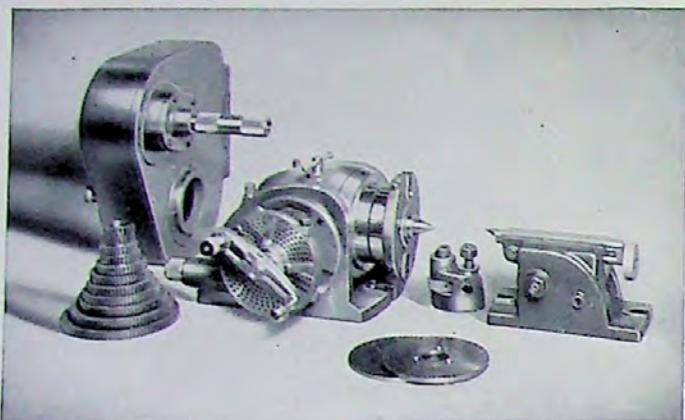
The exceptionally heavy spindle is mounted on anti-friction bearings to provide lasting accuracy. Accurate, long-time operation is assured. Large diameter swivel bearings, with means for locking securely at any angle, provide definite rigidity for severest conditions of operation.
