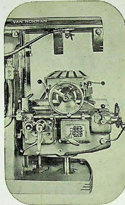
Front and rear directional power controls and hand feeds on models no. 3 standard and no. 2 heavy are at operator's finger tips . . . exclusive Van Norman single lever feed selector is reached easily from either operating position.
