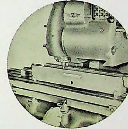
Vertical milling • Operator completes job with recess milling operation, using front controls. One work setup with simple changes in versatile cutterhead completes most jobs.
