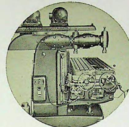
Adjustable cutterhead and movable ram in combination with the saddle crossfeed provide maximum milling capacity and versatility.
