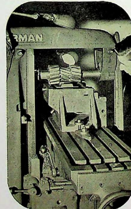
The typical gang milling operation is being performed on the Van Norman Horizontal Miller. The exceptionally rigid construction assures maximum accuracy under every type of cut.
