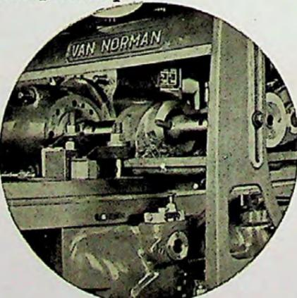
Horizontal setup for boring and facing operation. The ram-type overarm with dovetail ways and outer support assures rigidity and accuracy.
