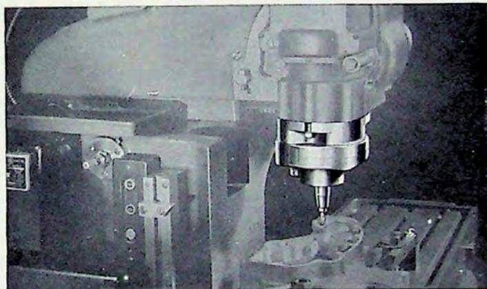
On high-speed work requiring a small diameter cutter, the Gear Type High Speed Attachment gives Van Norman Ram-Type Millers no. 22L, no. 26 and no. 36 added adaptability to perform such operations with fewer changes in setup.
