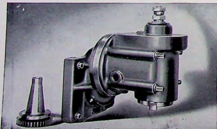
This attachment provides facility for adapting Van Norman Horizontal models of Milling Machines for vertical work. The unit is exceptionally heavy duty in construction, having a large diameter spindle with no. 50 National standard taper.
