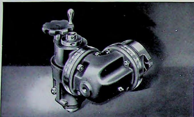
The spindle of this attachment is mounted in a compound swivel element which permits boring, drilling and milling at any angle—a feature invaluable in toolroom, experimental laboratory, and machine shop operation. Spindle quill unit has adjustment of 2½ in. operated by hand wheel actuating screw feed.
