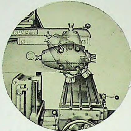
Adjustable cutterhead permits vertical, horizontal or angular milling, all on one Van Norman Ram-Type Miller . . . gives the work range of several single-purpose machines.
