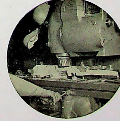
The ram-type miller used with adjustable cutterhead in the vertical milling position . . . operator using front directional controls.
