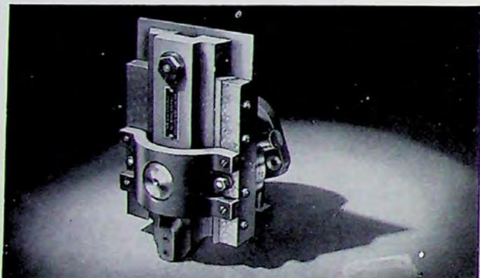
For giving clearance to dies, broaching, spline and keyway cutting, this attachment gives Van Norman Millers added range of capacity. With rigid construction and generously proportioned slide ways, it is operated on a 2 in. fixed stroke. Can be swiveled 360°. On ram-type models, in combination with adjustments of main cutterhead, slotter can be positioned to cut at any angle desired. Slotting head is bored to take round shank slotting tools.
