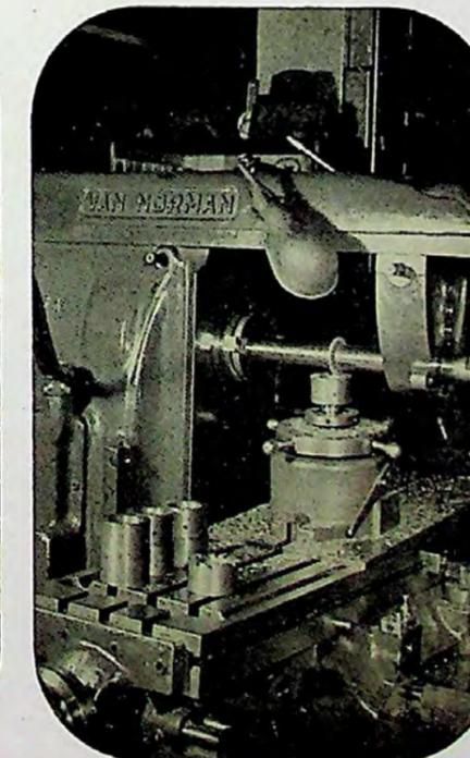
Precision milling of clutch jaws on the Van Norman Horizontal Miller. An indexing fixture is used for positioning the work for each cut.
