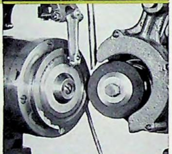
Grinding back radial surface of automotive differential pinion.
