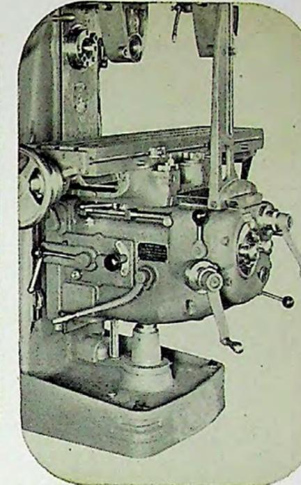
Central location of front and rear operating levers with positive directional control . . . fast selection of feeds . . . adjustable spindle clutch lever—all give ease of operation of no. 2 medium and no. 2 light duty millers.
