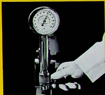
Bed ways are as hard as hardened steel . . . 70 to 72 Shore.
