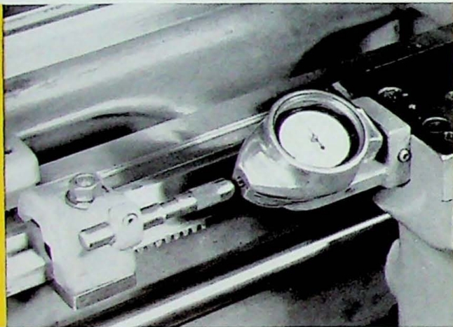
INDICATOR CARRIAGE STOP —Used when a facing or shoulder cut must be held within close limits. Precision type dial indicator, graduated in thousandths.
