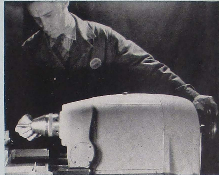
Drawbar Collet Attachment—Collets up to 1" are accurately centralized by the spindle nose mounted adaptor.
