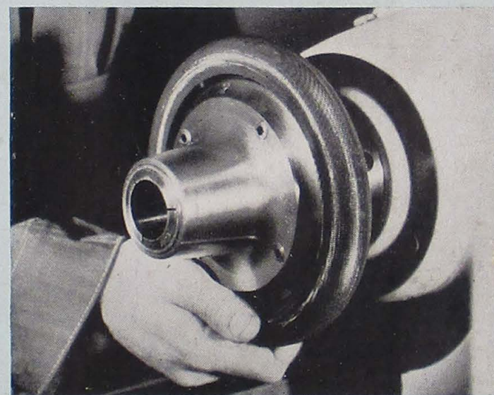
Sjogren Handwheel Collet Chuck—Fits directly to the Cam-Lock spindle nose and has collet capacity of 1 3/8" maximum.
