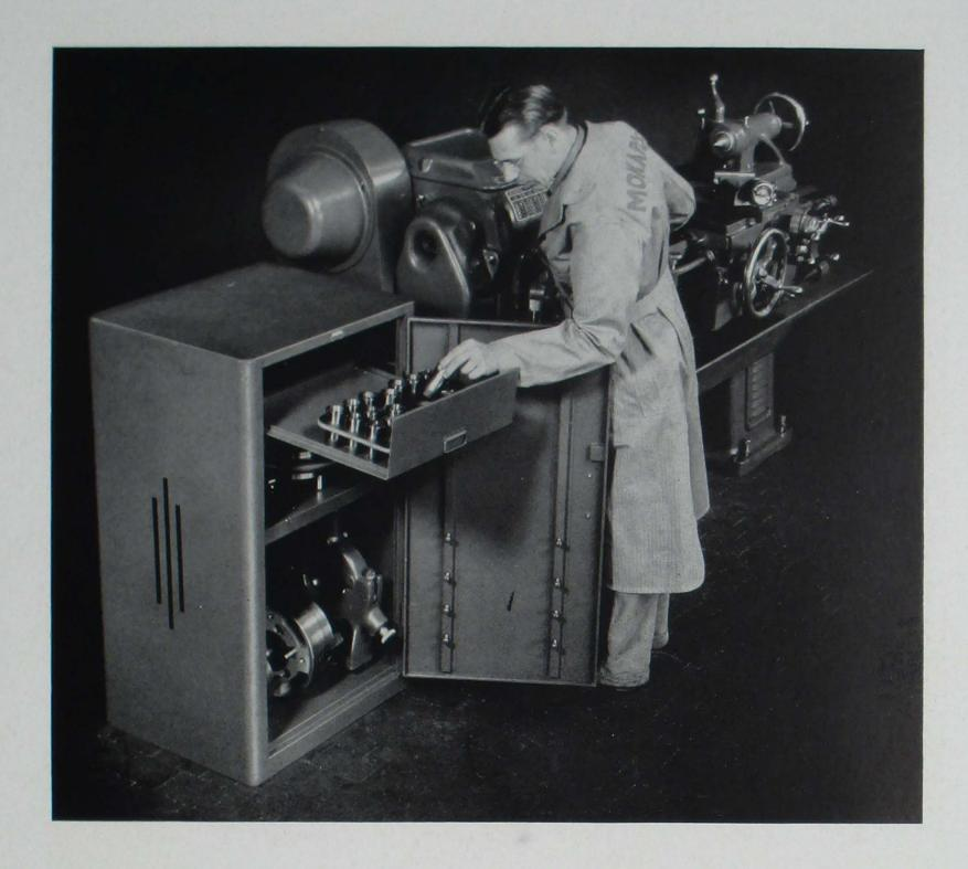
This tool cabinet was especially designed to provide proper storage space for the various accessory units normally used with each toolroom lathe. Made entirely of steel, this tool cabinet is 24" wide, 20" deep and 41" high. Space is provided in the top drawer for the storage of collets. Storage space is provided in the bottom of cabinet for such accessories as chucks, steady rest, follow rest, face plate, relieving attachment, as well as change gears for the relieving attachment.
