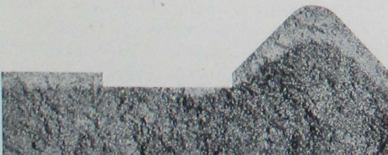
Above. Unretouched illustration of an etched "V" and flat way bed cross section after flame hardening. All Monarch sales offices have actual sections available for your examination.
