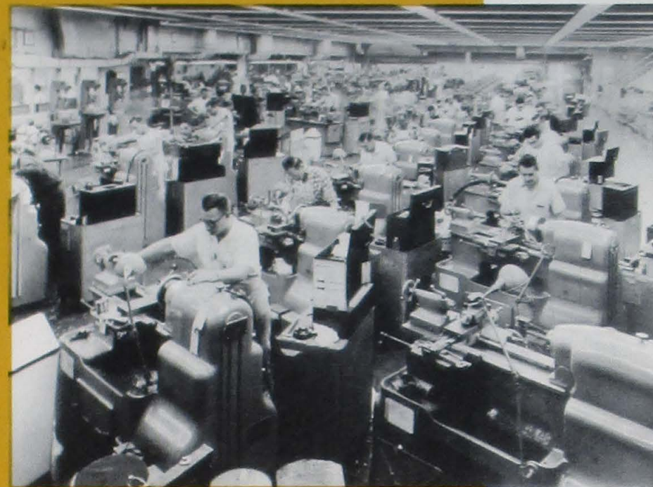
A battery of Model EE lathes, carefully chosen for their speed and precision, working on complex electronic equipment parts.
