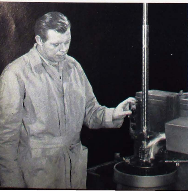
Below. Induction hardening the cross-feed screw for a Series 61 lathe.
