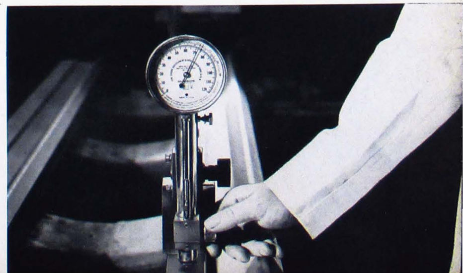
Above. Bed ways are ground to a tolerance of .0005 of an inch overall. Below. Bed ways are as hard as hardened steel—70 to 72 Shore.
