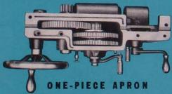
One-piece with double walls which carry rack-pinion, rack-wheel, and handwheel on anti-friction bearings. This construction maintains accurate alignment under excessive strains. Positive jaw feed clutch with single lever for both cross and length feed. All bearings in the apron, cross slide, and the front and rear ways of the bed are lubricated by a positive "one-shot" system.
