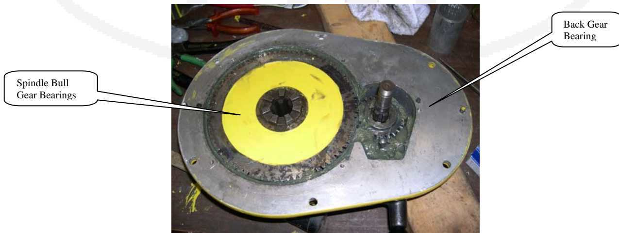
Figure 10 - Drive Housing Inspection
