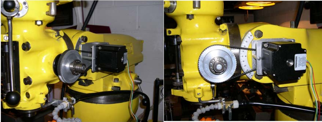
Figure 62 – Z Axis Installation
