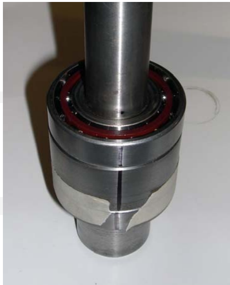
Figure 19 - Note the alignment marks on outer races preparing for next step
