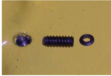
Figure 4 - Grub Screws, note the hollow locking screw.
