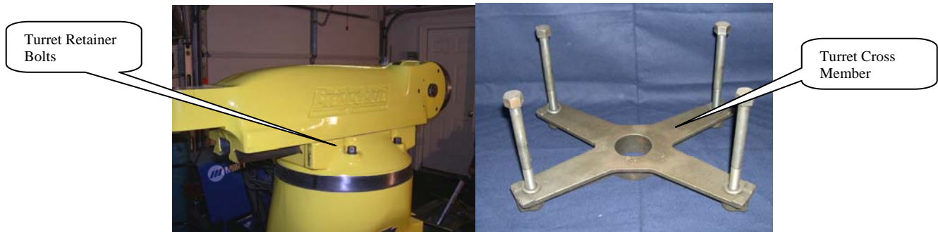
Figure 31 - Turret Bolts and Cross Member
