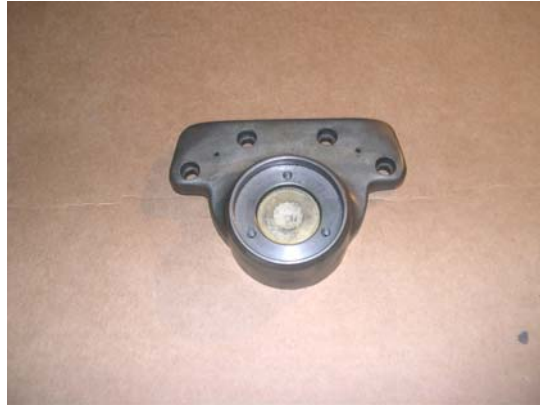
Figure 36 - Bearing Bracket with Bearings Installed
