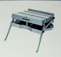
Combination sine tables — which allow setting up compound angles — and plain sine tables are available in 5 and 10" sizes (127 and 254mm). These tables are flat and square within .001".
