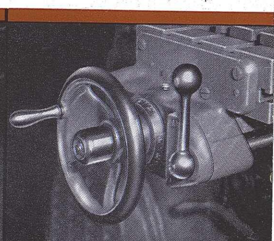
The Feed Selection Dial permits a choice of 32 feeds ranging from \frac{1}{4} to 60 inches per minute. Feeds range in approximate geometric progression with only one-half revolution of the lever required to increase or decrease the feed one step.
