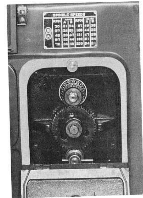
Fig. 75. Spindle speed pick-off gear box
