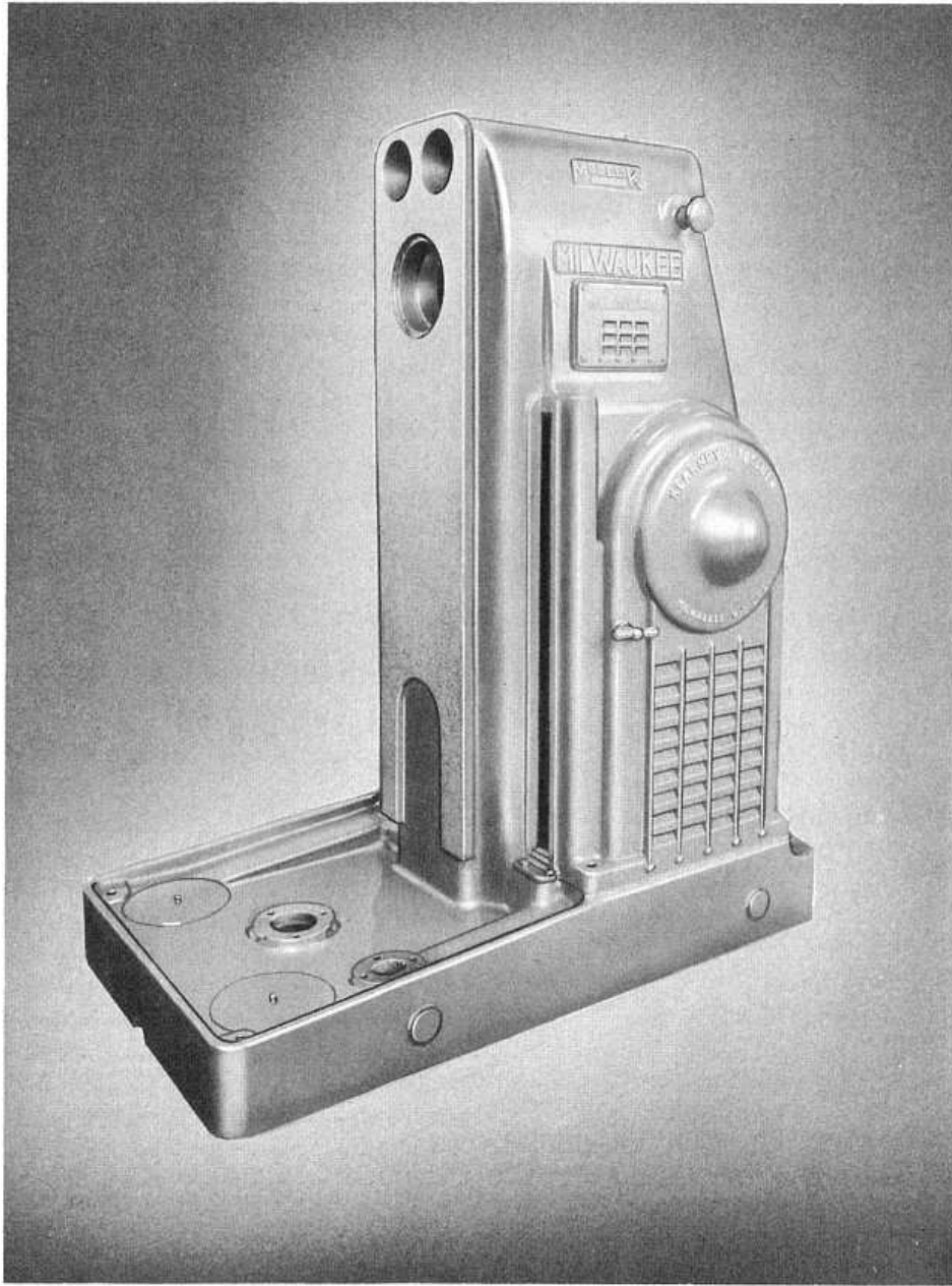
Fig. 2. The column — foundation of a milling machine
