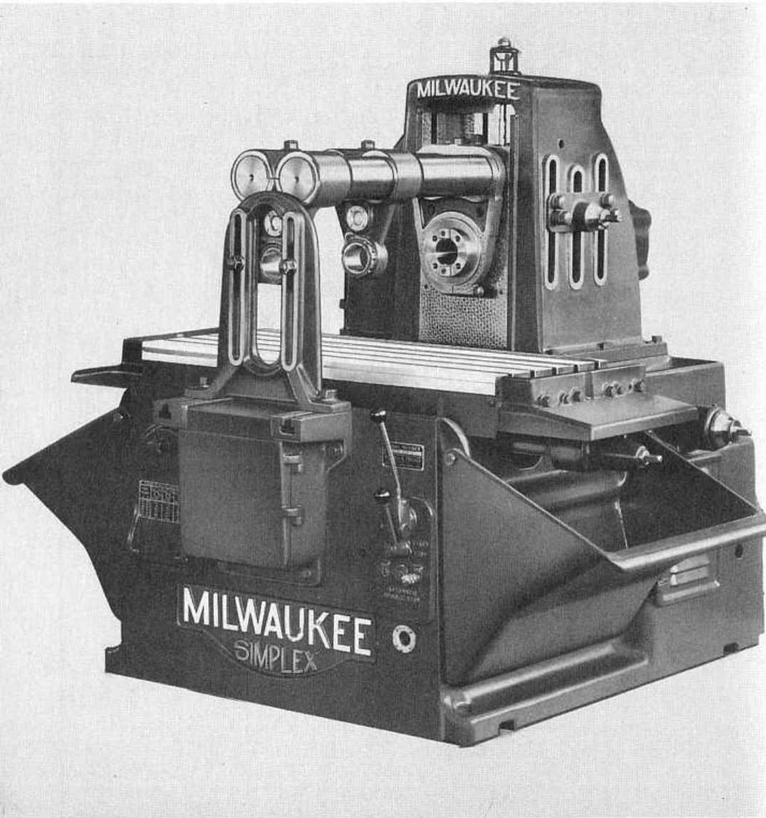
Fig. 14. Simplex bed-type milling machine
