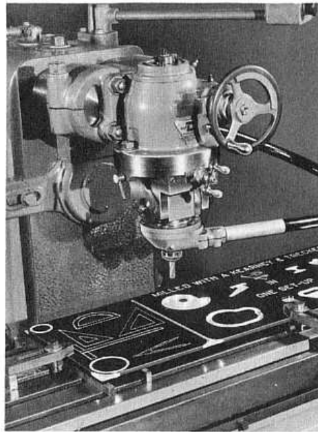
Fig. 22. Tri-D milling head on plain machine.
