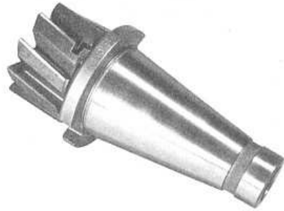
Fig. 65. Shell end mill mounted on style C arbor
