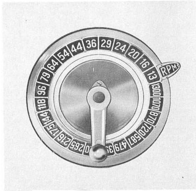
Fig. 4. Spindle speed selector dial and lever
