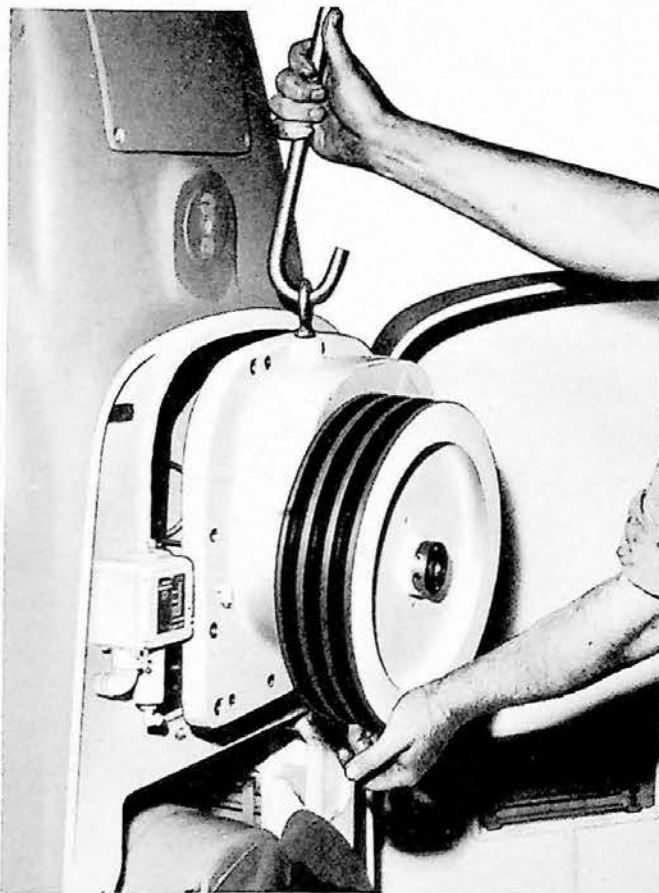
FIGURE 23A Removing Pulley Bracket
