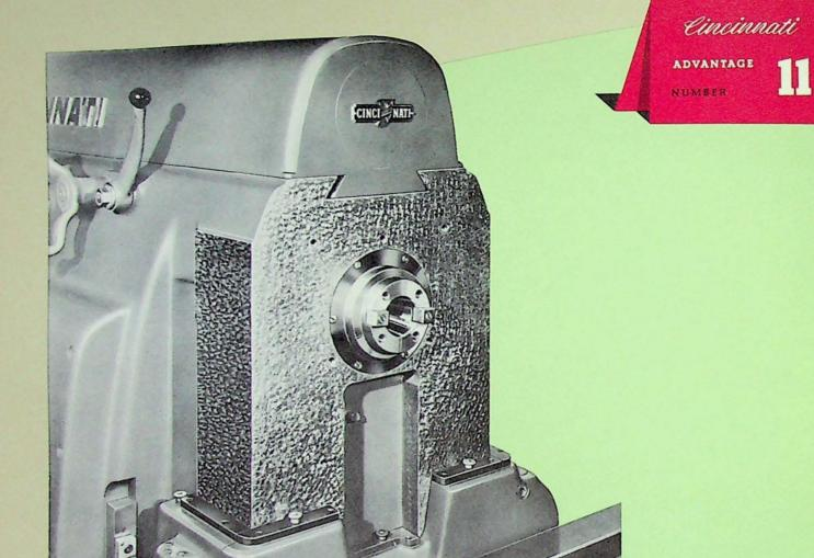
Look at the wide square gibbed grip the knee has on the column. It easily resists the stresses developed when taking heavy cuts with large cutters.
